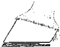
FIG. 104.—SHOE WITH A 'DROPPED' HEEL.
