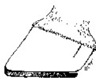
FIG. 93.—THE BEARING 'EASED' BY 'SPRINGING' THE HEEL OF THE SHOE.
