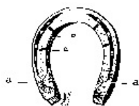
FIG. 76. This figure illustrates the principle of the Hartmann expanding shoe. a, a , The clips to catch the inside of the bars; b, c , saw-cuts.
