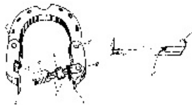
FIG. 73.—SMITH'S EXPANSION SHOE SEEN FROM ITS GROUND SURFACE AND FROM THE SIDE. a , The screw, with a fine-cut thread; b , nut which travels along it; c , a hollow thimble into which the screw passes at one end, the other being cut out V-shaped to catch into a slot ( d ) on the shoe; e, e , the grip[A] for the bars, the length and direction of which depend upon the shape of the foot; f, f , the counter-sunk rivets forming the hinge ( f' ); g , the counter-sunk rivet of the expanding piece.
