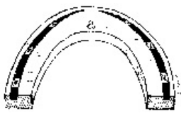
FIG. 110.—UNDER SURFACE OF THE TOE OF A HIND-SHOE. a , Marks the portion of the inner margin that inflicts overreach.
