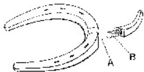
FIG. 108.—COLONEL NUNN'S SHOE WITH DETACHABLE TOE EXTENSION.
