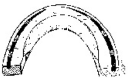
FIG. 111.—THE INNER MARGIN OF THE INFERIOR SURFACE OF THE HIND-SHOE BEVELLED TO PREVENT OVERREACH.
