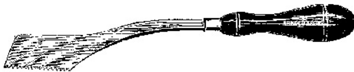
FIG. 144.—SMITH'S SIDE-BONE SAW (EARLY PATTERN).
