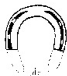
FIG. 63.—TIP SHOE. The dotted portions represent the length of the branches removed.
