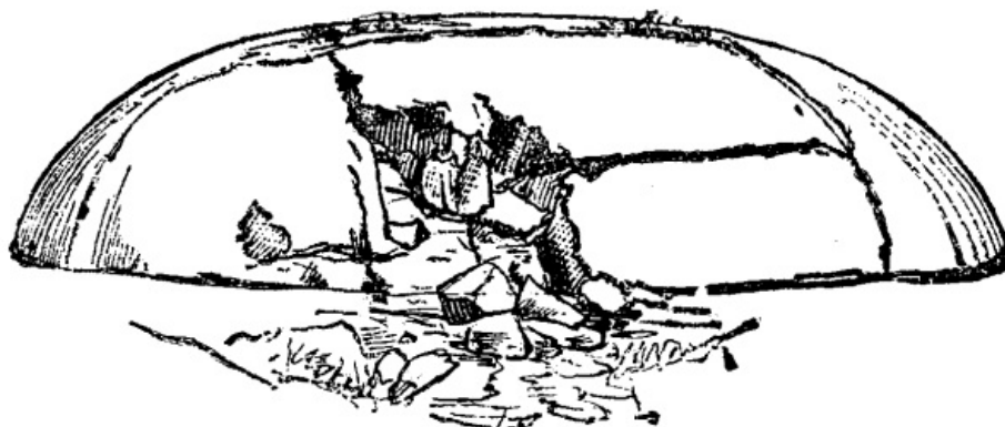
FIG. 4--STATE OF A CUPOLA AFTER THE ACTION OF THIRTY-SEVEN 6 IN. PROJECTILES.
