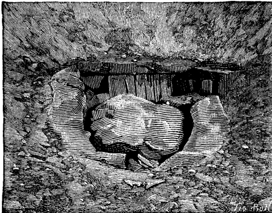
FIG. 7.--CASEMATE OF CHILLED IRON AFTER RECEIVING NINETY-SIX SHOTS.
