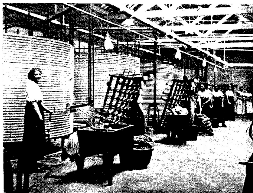
FIG. 27 A ROW OF MODERN WARPING MILLS
