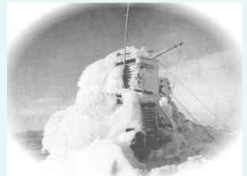
The Fergusson Metrograph on the summit of Mt. Rose, wrecked by snow "feathers," some of which were six feet long. Click photo to see full-sized.
