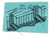
Approximately one-quarter of the total basement ceiling should be reinforced with extra joists and shielding material.
