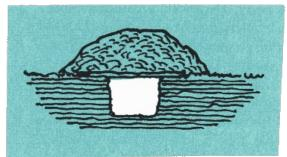
A fallout shelter, therefore, does not need to be a special type of building or an underground bunker. It can be *any space*, provided the walls and roof are thick or heavy enough to absorb many of the rays given off by the fallout particles outside, and thus keep dangerous amounts of radiation from reaching the people inside the structure.
