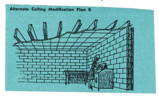
This is similar to Plan A, except that new extra joists are fitted into part of the basement ceiling to support the added weight of the shielding (instead of using a beam and a screwjack column).
