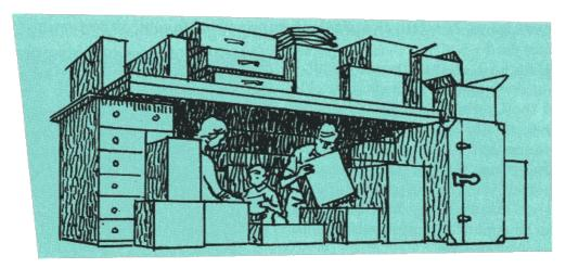
With doors, furniture and appliances, plus stacks of other shielding material, you can create an enclosure large enough to live in for a short time. If possible, use boxes filled with sand or earth
