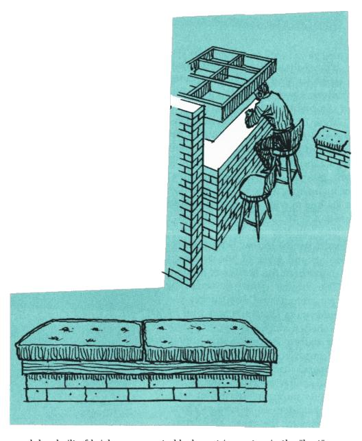
This is a snack bar built of bricks or concrete blocks, set in mortar, in the "best" corner of your basement (the corner that is most below ground level). It can be converted quickly into a fallout shelter by lowering a strong, hinged "false ceiling" so that it rests on the snack bar.
