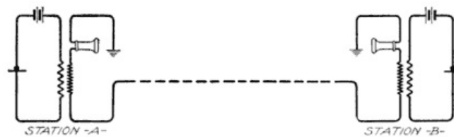
Fig. 125. Local-Battery Stations with Grounded Circuit
