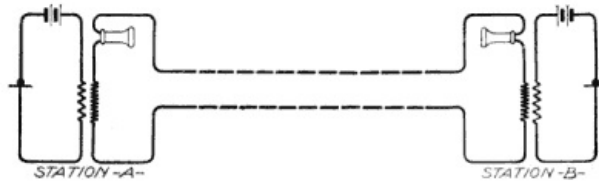
Fig. 126. Local-Battery Stations with Metallic Circuit View full size illustration.
