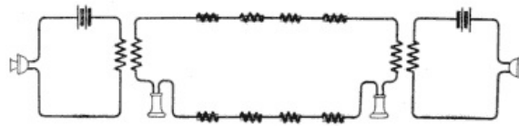
Fig. 34. Test of Line with Varying Serial Inductance View full size illustration.
