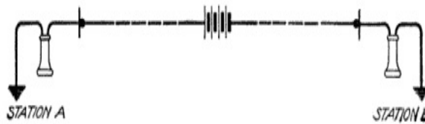
Fig. 128. Battery in Series with Two Lines View full size illustration.
