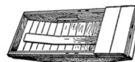
Fig. 63. Nailing on the Decks.
