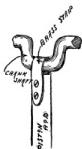
Fig. 294. Connection of Rod and Crank.
