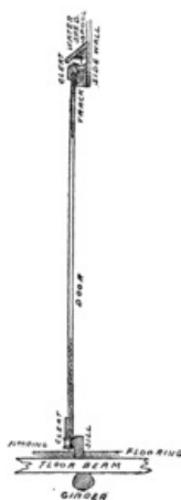
Fig. 144. Section of the Door and Frame.
