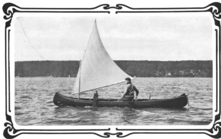
The Indian Canoe Fitted with Lanteen Sail and Lee Boards.
