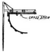
Fig. 122. Section of the Canoe, Showing Lee Board.
