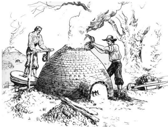
MAKING "TRIALS" OF IRON. EVIDENCES OF AN EARTH OVEN OR SMALL FURNACE WERE DISCOVERED AT JAMESTOWN DURING ARCHEOLOGICAL EXPLORATIONS. SMALL AMOUNTS OF IRON MAY HAVE BEEN SMELTED IN THE FURNACE DURING THE EARLY YEARS OF THE SETTLEMENT. (Conjectural sketch by Sidney E. King.)
