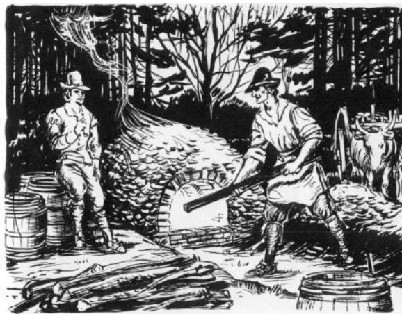
MAKING LIME FROM OYSTER SHELLS IN A KILN, ABOUT 1625. (Conjectural sketch by Sidney E. King.)
