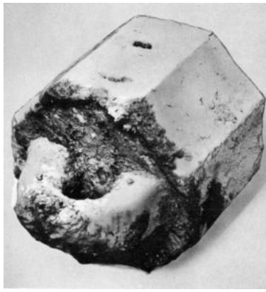
THIS 1,300-POUND IRON PILEDRIVER USED FOR DRIVING PILES IN THE BUILDING OF SMALL WHARVES WAS FOUND AT JAMESTOWN.
