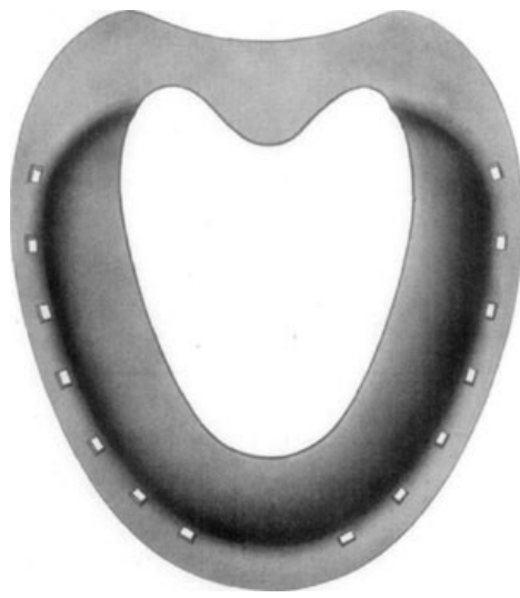
Fig. 36—Superior surface, showing concavity or bowl, as formed by the toe and branches of the shoe, as designed by Dr. David W. Cochran.
