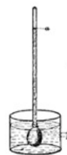
FIG. 2.—In the bladder A is a sugar solution. In the vessel B is pure water. Sugar passes out and water into the bladder until it rises in the tube to a .
