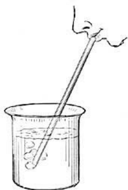
FIG. 145.—Water does not enter the tube as long as we blow into it.
