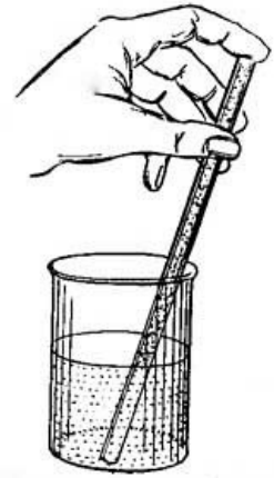
FIG. 42.—Water rises in the tube when the air is withdrawn.
