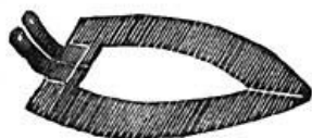
FIG. 202.—The fine wires are strongly heated by the current which flows through them.
