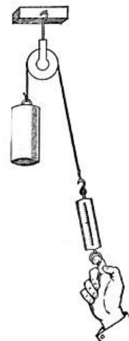
FIG. 109.—By means of a pulley, a force in one direction produces motion in the opposite direction. [168]
