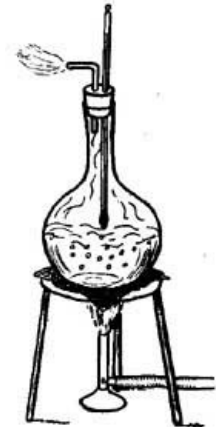
FIG. 9.—Determining one of the fixed points of a thermometer.
