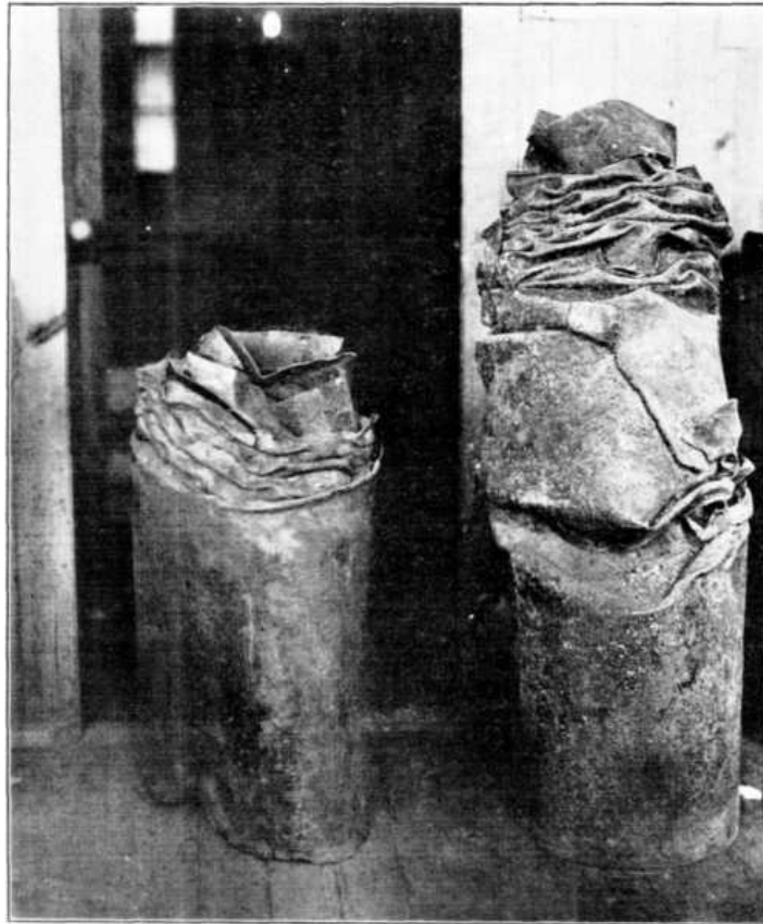
PLATE XXIX, FIG. 1.—A 14-GAUGE, 14-IN., HOLLOW (NON-TELESCOPIC), CALIFORNIA STOVE-PIPE PILE WHICH MET IMPENETRABLE MATERIAL.
