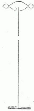
Salmon weir, Bucksport. Leader, brush, 4 to 8 rods long. Middle pond, 40 feet long, 8-foot entrance; inner side, brush; outer side, twine. Pockets, twine, 10 feet long, 10-inch entrances, wooden floor. Value, $25. Some weirs have only one (upstream) pocket.
