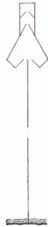
Salmon weir, Stockton. Leader 200 feet long; brush from shore to low-water mark; remainder brush at bottom, netting at top. Head 60 feet long; outer pound 40 feet, middle pound 12 feet, inner pound 8 feet; brush below low-water line, netting above; plank floors in two smaller compartments. Value, $40.
