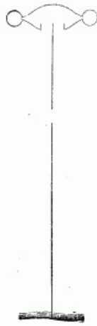
Salmon weir, Winterport. Leader, brush, 6 rods long. Heart, brush or netting, 40 feet long, 20 feet wide, with 8-foot entrance on each side of leader. Pockets, netting, 10 feet in diameter, 9-inch entrance, wooden floor. Value, $50.
