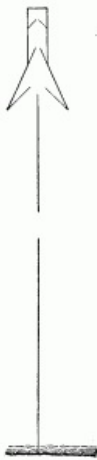
Salmon weir, Castine. Hedge 200 feet long, made of stakes driven in mud interwoven with brush to low-water mark, covered with netting beyond. Great pound, 30 feet long, 30 feet wide at base, made of netting; entrance 8 feet wide. Inner pounds, 10 feet wide, with board floors; outer entrance 2 feet wide, inner 1 foot. Value, $70.
