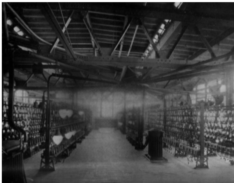
ON THE TESTING-RACKS OF THE MANUFACTURER OF INCANDESCENT FILAMENT LAMPS
