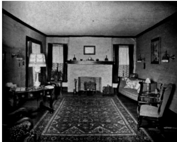
OBTAINING TWO DIFFERENT MOODS IN A ROOM BY A PORTABLE LAMP WHICH SUPPLIES DIRECT AND INDIRECT COMPONENTS OF LIGHT
