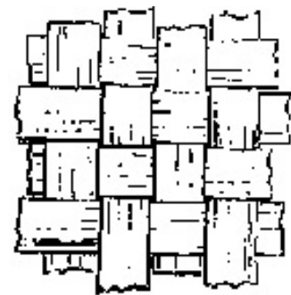
FIG. 293. Surface relief produced by wide fillets set close together.
