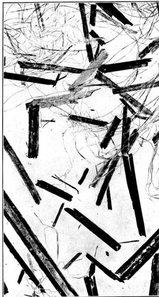
FIG. 3.—A representative sample of hemp hurds, natural size, showing hemp fiber and pieces of wood tissue.
