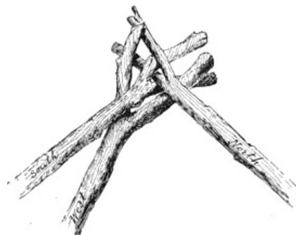
FIG. 230—The three main timbers of a hogán
