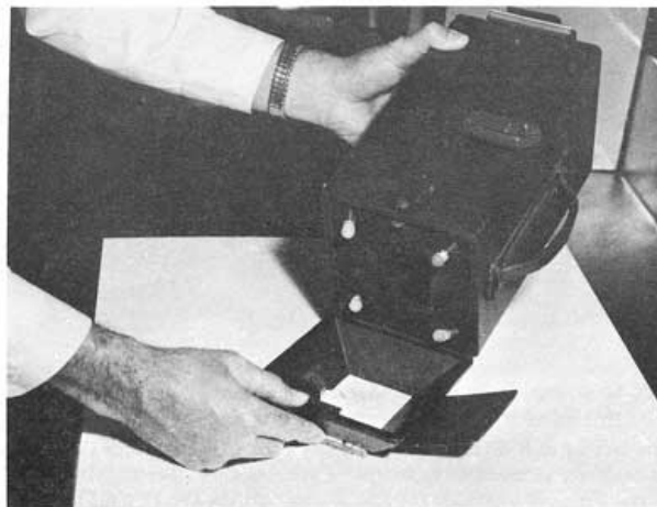
427. Centering of latent in aperture insures equal distribution of light over print.
