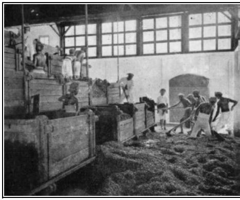
FERMENTING BOXES, JAVA. From the last box the beans are shovelled into the washing basin. (Reproduced from van Hall's Cocoa , by permission of Messrs. Macmillan & Co.)
