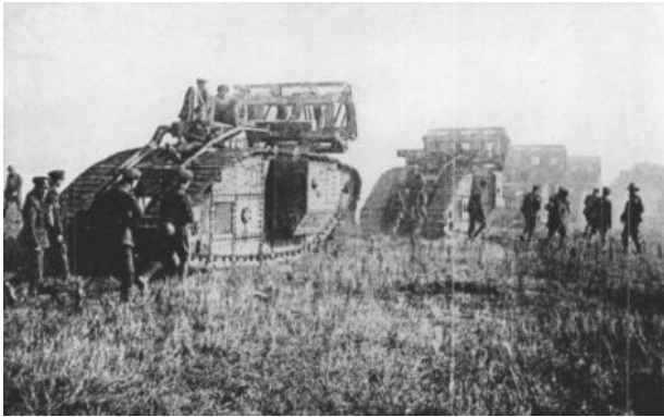
BRITISH TANKS ADVANCING ACROSS THE HINDENBURG LINE. This battery of tanks shows the new superstructure on their fronts, which is used to carpet the slippery mud which the caterpillar wheels do not grip.
