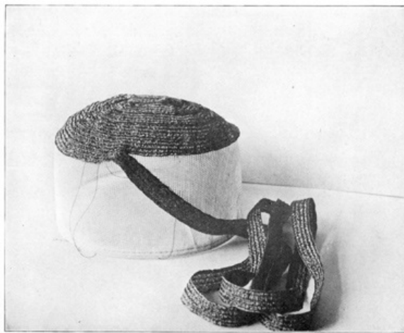
ONE METHOD OF STARTING THE BRAID ON CROWN AND SEWING IN PLACE
