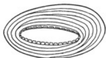
BRAID-COVERED BRIM SHOWING METHOD OF FILLING IN SHORT LENGTHS WHEN THE DIFFERENCE IN WIDTH OF THE TWO SIDES IS VERY GREAT
