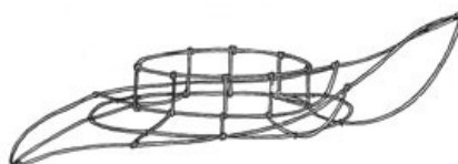
ROLLING WIRE BRIM. EIGHT SPOKES MORE MAY BE USED AND AS MANY CIRCLES AS WISHED, ACCORDING TO THE COVERING USED
