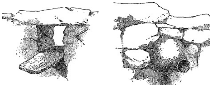
FIG. 43. Tusayan roof drains; a discarded metate and a gourd.
