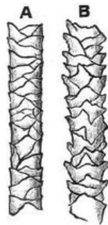
FIG. 4.—Showing the Effects of Scouring Agents on the Wool Fibre. A. Unscoured Fibre. B. Badly Scoured Fibre.
