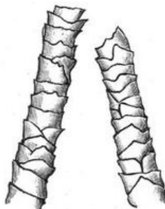
FIG. 5.—Wool Fibre Heated with Acid.
