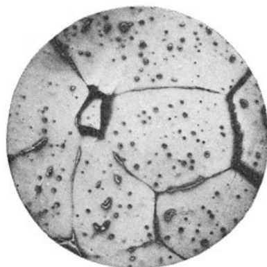
FIG. 49.—Coarse-grained martensite, polished and etched with nitric acid and magnified 50 times. Made by Prof. Chas. Y. Clayton.
