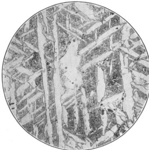
FIG. 69.—A portion of 67 magnified 200 diameters, showing that pearlite areas are no longer laminated and providing reason for observed hardness
