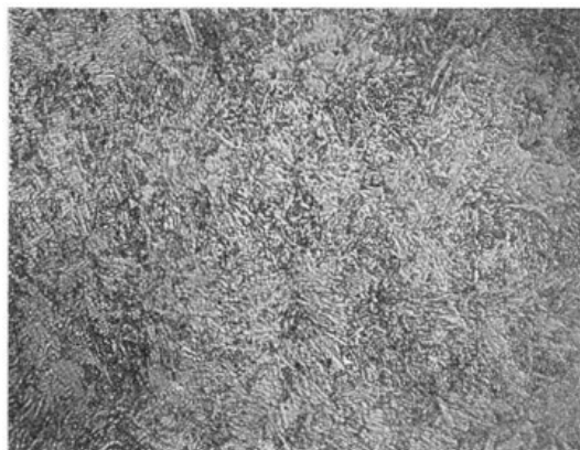
FIG. 50.—Quenched high-carbon steel, polished, etched and viewed at 100 magnifications. This structure is called martensite and is desired when maximum hardness is essential. Photograph by H. S. Rawdon.
