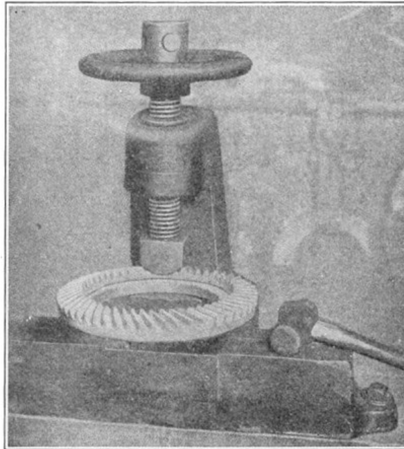
FIG. 57.—Press for holding test gears for breaking.
