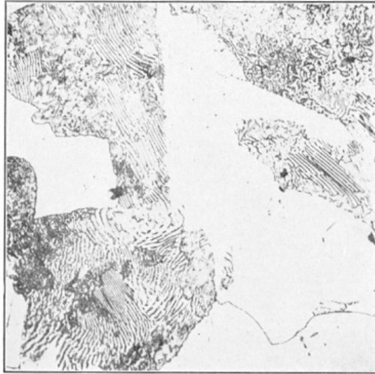
FIG. 77.—Peg withdrawn after cooling to 670°C. (magnified 800 diameters). Just at this moment the lamination of pearlite, which now occupied its original area, was taking place. In some parts the lamination was perfect, in other parts the iron and iron-carbide were still dissolved in each other.
