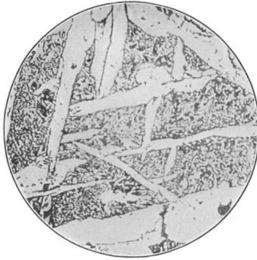
FIG. 70.—Peg withdrawn at 780°C. (magnified 25 diameters), showing inter-diffusion of transformed pearlite and ferrite areas.
