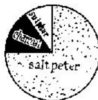
FIGURE 16—GUNPOWDER. Black powder (above) is a mechanical mixture; modern propellants are chemical compounds.
