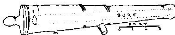
FIGURE 27—SPANISH 24-POUNDER CAST-IRON GUN (1693). Note the modern lines of this cannon, with its flat breech and slight muzzle swell.
