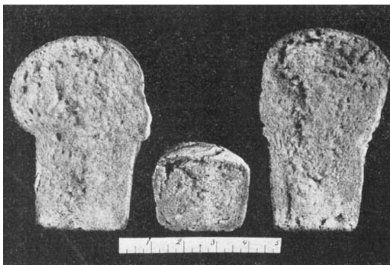
FIG. 49.—BREAD FROM NORMAL FLOUR (1); GLIADIN EXTRACTED FLOUR (2); AND FROM FLOUR AFTER EXTRACTION OF SUGAR AND SOLUBLE PROTEIDS (3).
