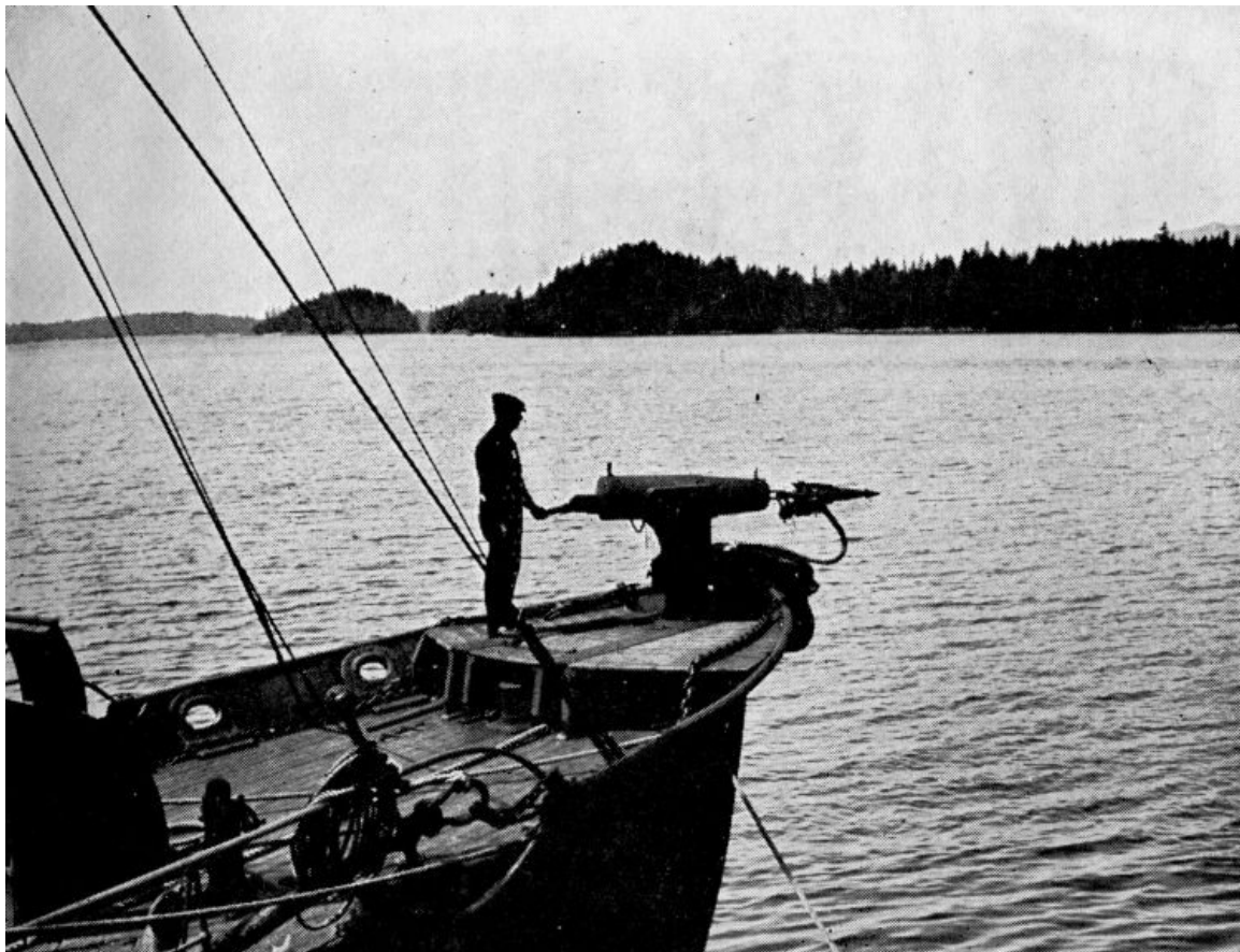
Whale Harpoon Gun loaded and being turned so as to point at the Whale.
