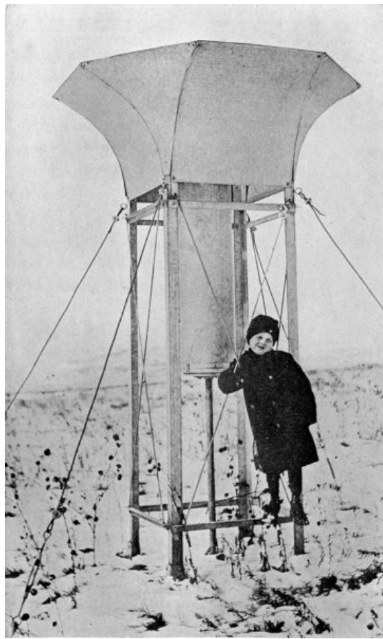
MEASURING THE BLIZZARD'S RAGE. Shielded snow gauge in the Northwest to register the amount of snow-fall.
