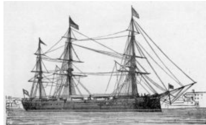
THE TURRET-SHIP "MONARCH," BATTLESHIP OF 1869. Length, 180 feet; Displacement, 6200 tons; Speed, 15 knots; Armament, 7 guns of 25 and 12 tons.
