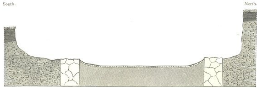
FIG. 14.—A north and south section through the subsided floor of a corridor, paved with tesserae. Outside the broken-down bounding walls, the excavated ground on each side is shown for a short space. Nature of the ground beneath the tesserae unknown. Silchester. Scale \frac{1}{32} .
