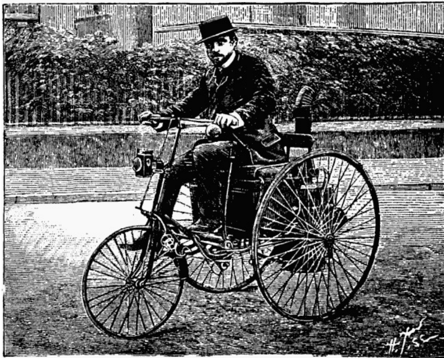
FIG. 2.—TRICYCLE PROPELLED BY A SERPOLLET BOILER
