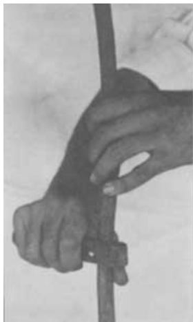
Fig. 2. First operation. Making parallel cuts on stock.]
