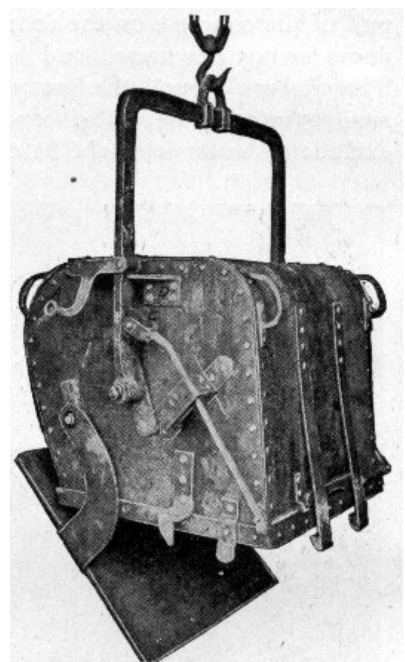
Fig. 28.—Cyclopean Bucket for Depositing Concrete
