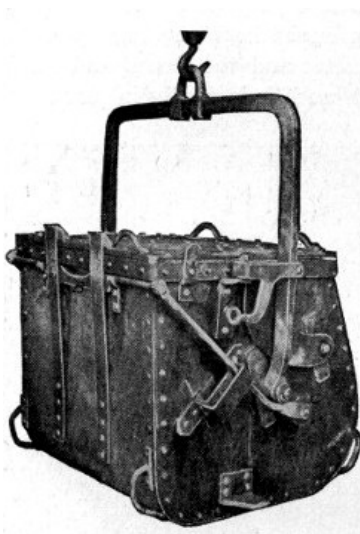
Fig. 27.—Cyclopean Bucket for Depositing Concrete Under Water (Closed Position).
