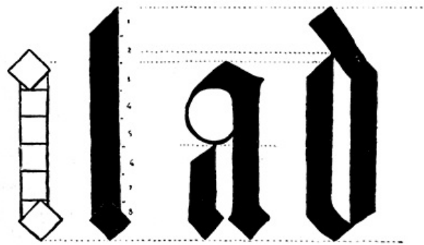
PROPORTIONS OF LOWER-CASE GERMAN TEXT AND METHOD OF DRAWING THE LETTERS (FROM ALBERT DÜRER'S "GEOMETRICA")
