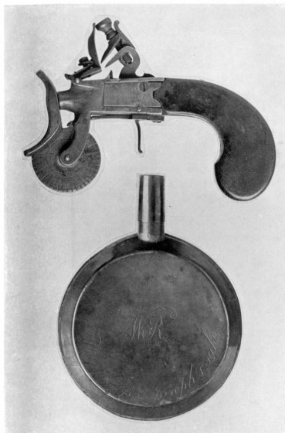
FIG. 92.—A POWDER TESTER. FIG. 93.—A PRIMING FLASK. (In the Municipal Museum, Hull.)
