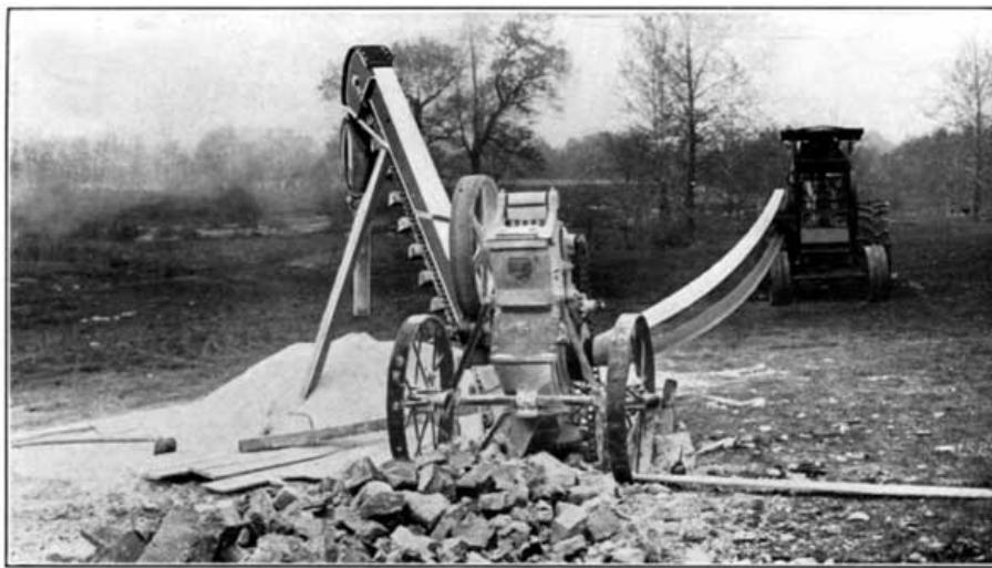
A Limestone Pulverizer for Farm Use (Courtesy of the Jeffrey Manufacturing Company, Columbus, Ohio)
