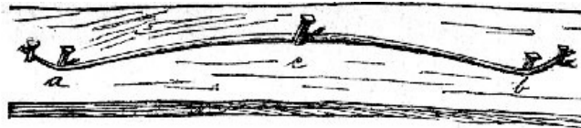
Fig. D. (A and B are six inches from the ends. The bow is bent slightly at C.)
