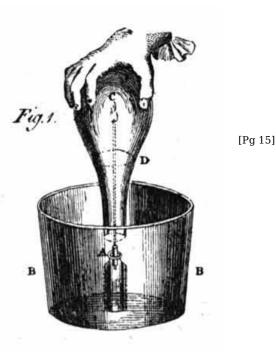
that case the external air resting upon the water seeks equilibrium again after the flask has become cold, and presses the same measure of water into the flask as of air had been previously driven out by the heat. Accordingly, I made the following experiment:
