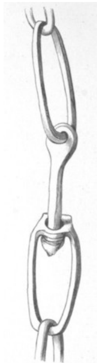
Fig. 78. Piece of chain, shewing the swivel: Hereford. Actual size.
