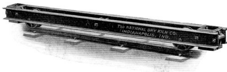
Fig. 81. A Regular Channel-iron Kiln Truck.
