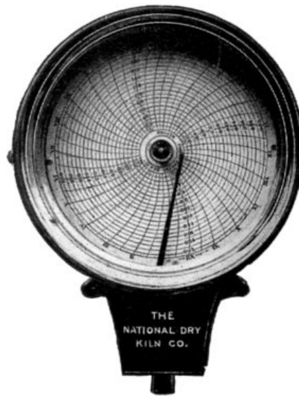
Fig. 99. The Recording Steam-Pressure Gauge.]
