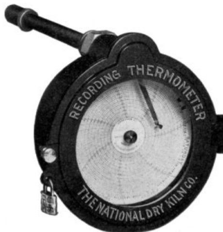
Fig. 97. The Recording Thermometer.
