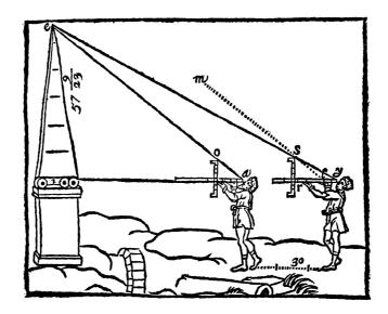
Let the first aime be taken from a, the beginning of the Index perpendicular unto the height to be measured: And from an unknowne length ai, by o, the end of the transome, unto e, the toppe of the height ei: And let the segment of the Index be ua. The second ayme, let it be taken from y, the beginning of the same Index; and out of a greater distance, by s, the end of the transome, unto the same toppe e. And the segment of the Index let it be  $\underline{ry}$ .
