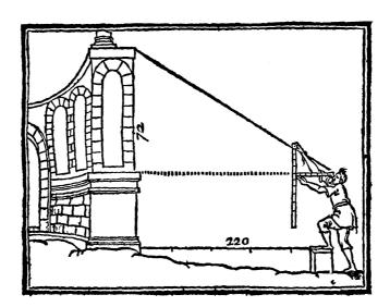
The Figure is thus: And the demonstration is by the 12 e vij, as afore: but here is to be added the height of the measurer; which if it be 4 foot, the whole height shall be 76 foote.
