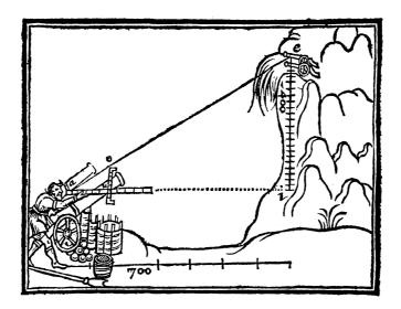
This is the first and second kinde of measuring of a Longitude, by one single distance or station: The third which is by a double distance doth now follow. Here the transome, if there be roome enough for the measurer to goe farre enough backe, must be put lower, in the second distance.
