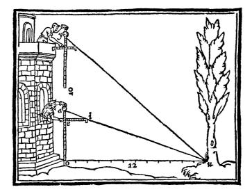
The same manner of measuring shall be used from an higher place; as out of y, the segment of the Index is 5. parts; the segment of the transome 6: and then the height be 10 foote: the same Length shall be found to bee 12 foote.
