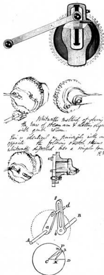
Figure 44.—Quick-return mechanism. Top , Early representation of the quick-return mechanism patented by Whitworth in 1849, from William Johnson, ed., The Imperial Cyclopaedia of machinery (Glasgow, about 1855, pl. 88). Middle , Sketch by Robert Willis from his copy of Principles of Mechanism (London, 1841, p. 264), which "shews Whitworth dissected into a simpler form"; it is as obscure as most subsequent attempts have been to explain this mechanism without a schematic diagram. Bottom , Linkage that is kinematically equivalent to Whitworth's, from Robert Willis, Principles of Mechanism (London, 1841, p. 264).
