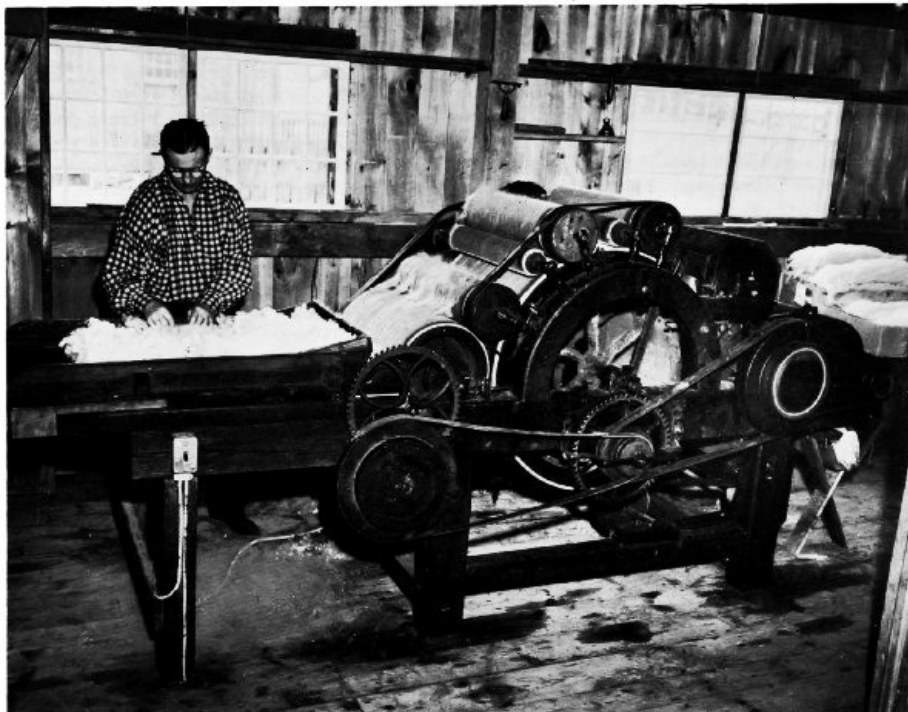
Figure 10.—AN ORIGINAL SCHOLFIELD WOOL-CARDING MACHINE AT OLD STURBRIDGE VILLAGE, STURBRIDGE, MASSACHUSETTS. It is now run by electricity. (Photo courtesy of Old Sturbridge Village.)
