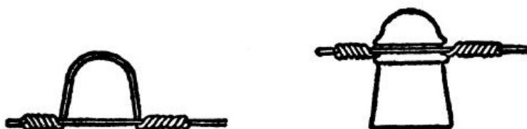
Transmission wire on glass insulator
