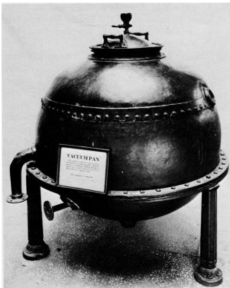
FIGURE 3.—Gail Borden's vacuum pan of 1853, used to make condensed milk. (Catalog No. 26.)
