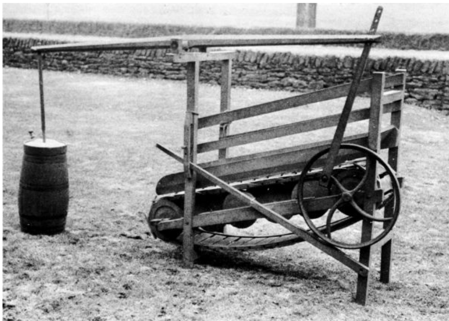
FIGURE 14.—Dog-powered churn, 1881. (Catalog No. 140.)
