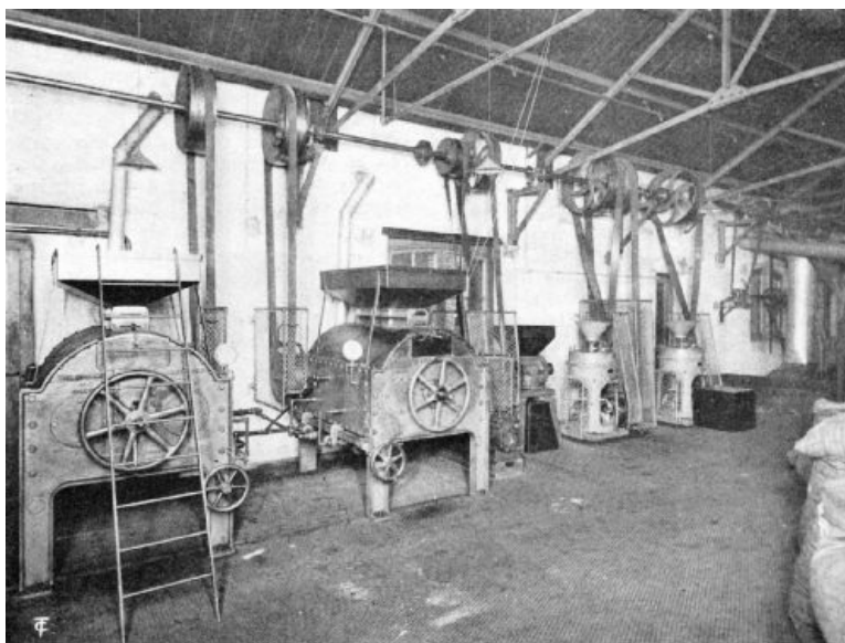
AN ENGLISH GAS COFFEE-ROASTING PLANT The machines are the Morewood (Improved Faulder) sliding-burner indirect type
