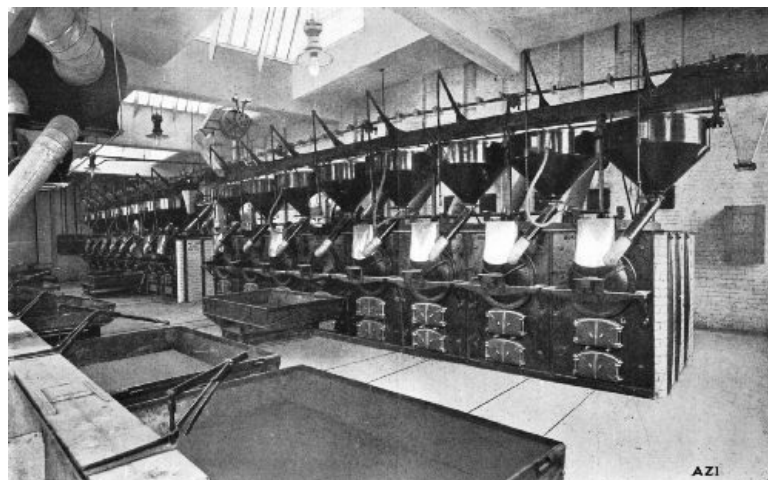
A SIXTEEN-CYLINDER COAL ROASTING PLANT IN A NEW YORK FACTORY
