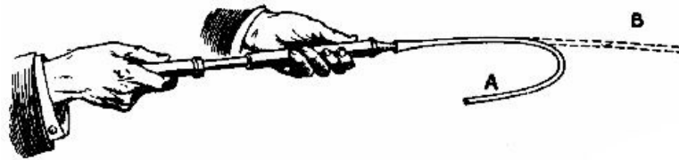
FIG. 13.—Showing the principle of the steam-gauge.
