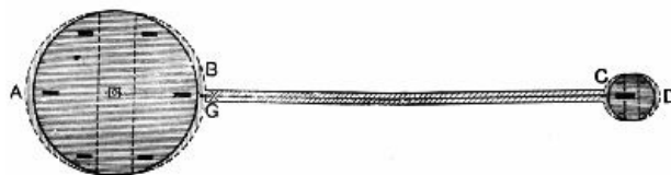
FIG. 111.—Earth and moon model, illustrating the production of statical or "equilibrium" tides when the whole is whirled about the point G.
