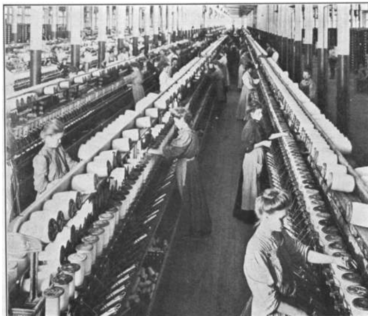
Each operator at these spoolers has a Barber knotter on her hand
