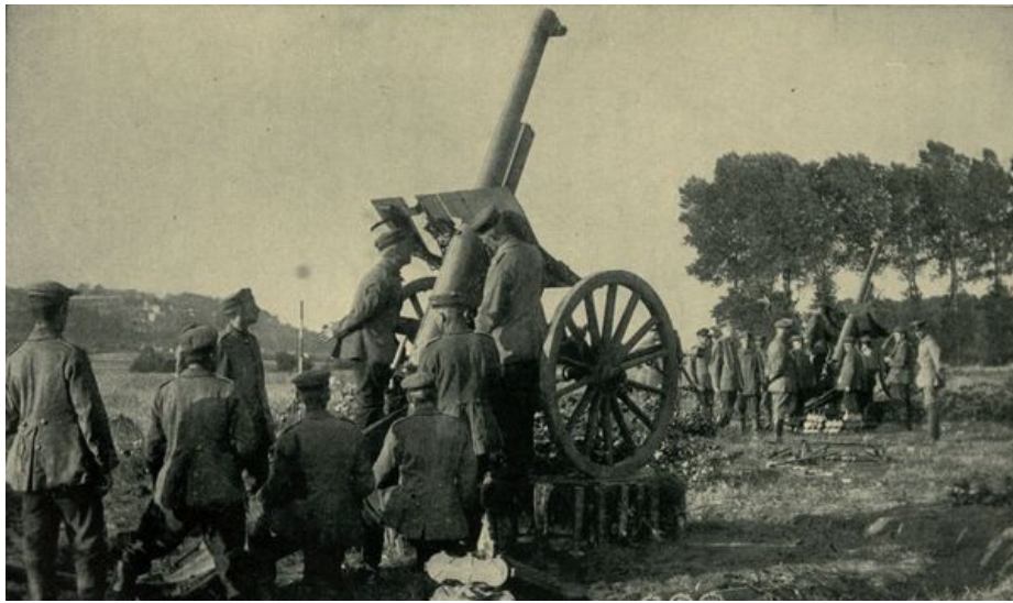
GERMAN AEROPLANE GUNS, MOUNTED ON TURNABLES. THEY CAN BE TURNED QUICKLY TO ANY DIRECTION AND TO WHATEVER ANGLE OF ELEVATION IS REQUIRED.
